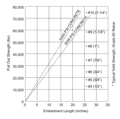
On-site tests should be carried out to verify anchorage performance of various steel components used with 21-30 Anchortite. The chart at left represents typical anchorages with grade 60 rebar in 3000 a n d 5 0 0 0 p s i unreinforced concrete, for threaded and deformed ½" to 1-¼" diameter bars.
